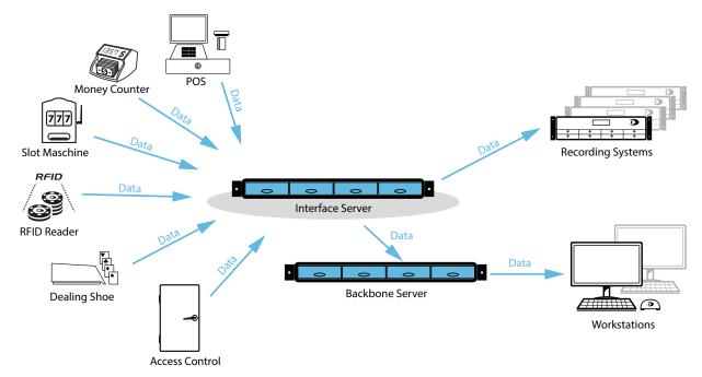
The HEMISPHERE® SeMSy® Interface Module provides an interface to external devices in a SeMSy® video management system. The module receives data from external devices (e.g. POS, access control, dealing shoe) via Ethernet and stores them in the integrated database. The received data can be processed and forwarded to various systems to trigger an action.
